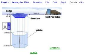
Diagram of IceCube. IceCube will occupy a volume of one cubic kilometer. Here we depict one of the 80 strings of opctical modules (number and size not to scale). IceTop located at the surface, comprises an array of sensors to detect air showers. It will be used to calibrate IceCube and to conduct research on high-energy cosmic rays. Author: Steve Yunck, Credit: NSF
