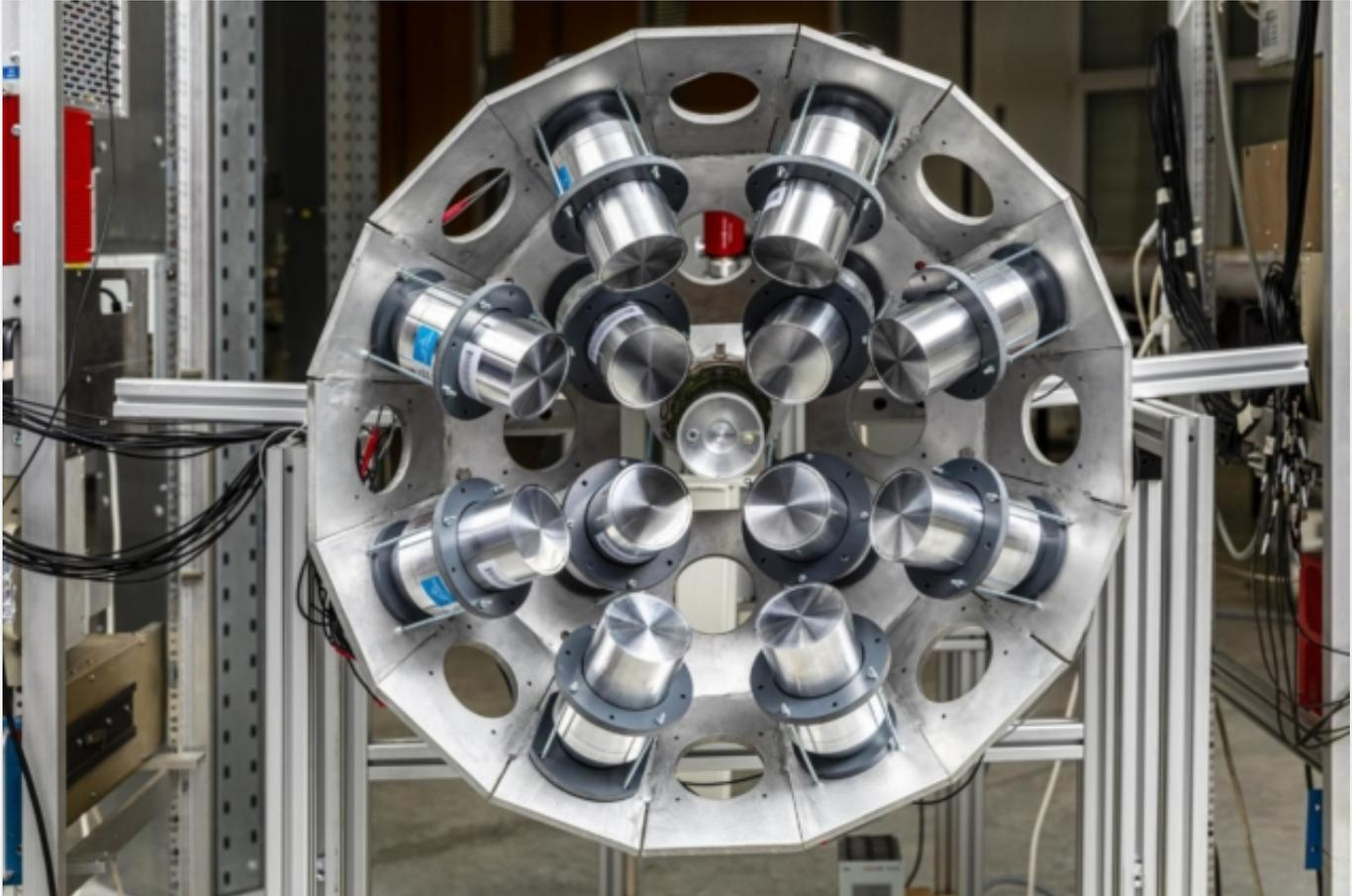
Atomki's new high-resolution  $\text{LaBr}_3$  spectrometer, which will record gamma–gamma pairs from excited nuclei. Credit: Atomki
