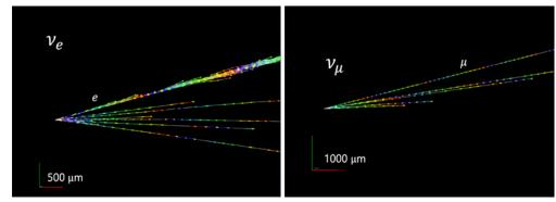
Event displays identified by the FASER collaboration as candidates for an ve (left) and a vµ (right) interacting in the detector. Invisible here, the neutrinos arrive from the left and then interact to create multiple tracks spraying out to the right (coloured lines), one of which is identified as a charged lepton (labelled). (credit: FASER collaboration)
