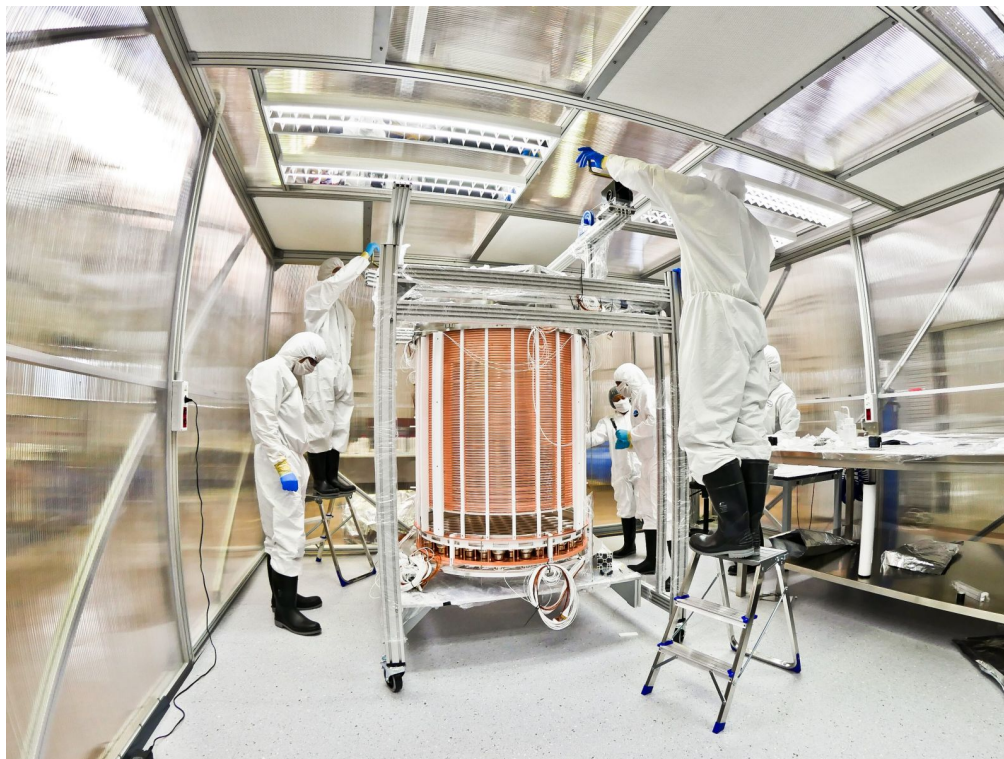
The XENON1T Time Projection Chamber (TPC) after assembly in a clean room. Photo: XENON1T
