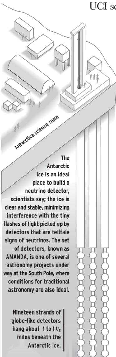
Nineteen strands of globe-like detectors hang about 1 to 1 1/2 miles beneath the Antarctic ice.
