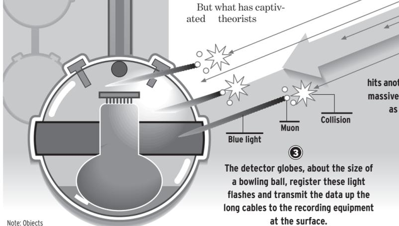
The detector globes, about the size of a bowling ball, register these light flashes and transmit the data up the long cables to the recording equipment at the surface.
