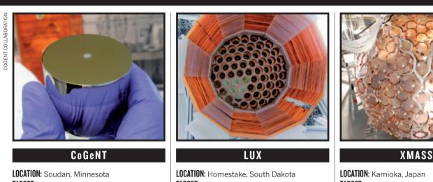
TARGET: 500 g germanium crystal MASS RANGE: <10 GeV START DATE: 2004 FINDINGS: Hundreds of detections TARGET: 350 kg liquid xenon MASS RANGE: 10-100 GeV START DATE: 2011 FINDINGS: Not yet started
