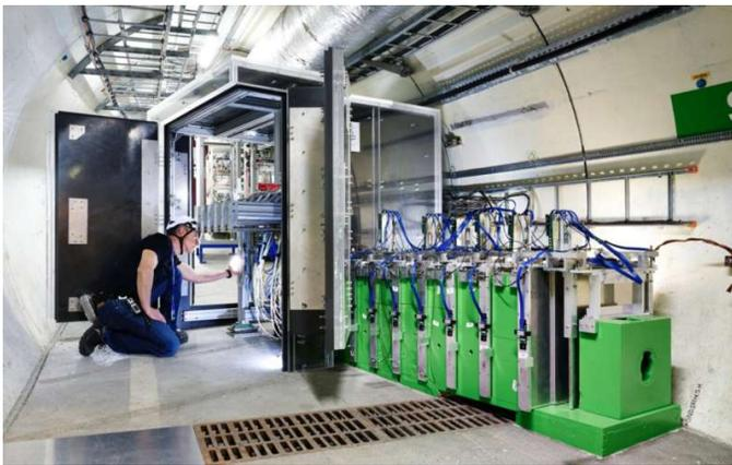
The new experiment SND@LHC installed at CERN's Large Hadron Collider. Neutrinos impinge on the detector from the left and interact in the target, on which the flashlight is being shone. Hadronic jets and muons produced in the neutrino interactions are measured by the experiment's calorimeter, which is painted in green. Credit: Brice, Maximilien; SND@LHC Collaboration.
