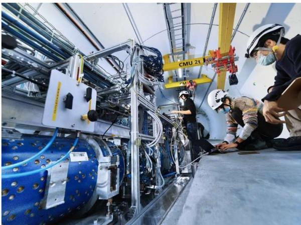
The final elements of the FASER (Forward Search Experiment) detector are installed in the T12 tunnel of the LHC. It is located along the beam collision axis, 480 m from the ATLAS interaction point, in an unused service tunnel that previously connected the SPS to the LEP collider. FASER began taking data in July 2022 at the beginning of LHC Run 3. Photograph: Maximilien, Brice; Ordan, Julien, FASER Collaboration.
