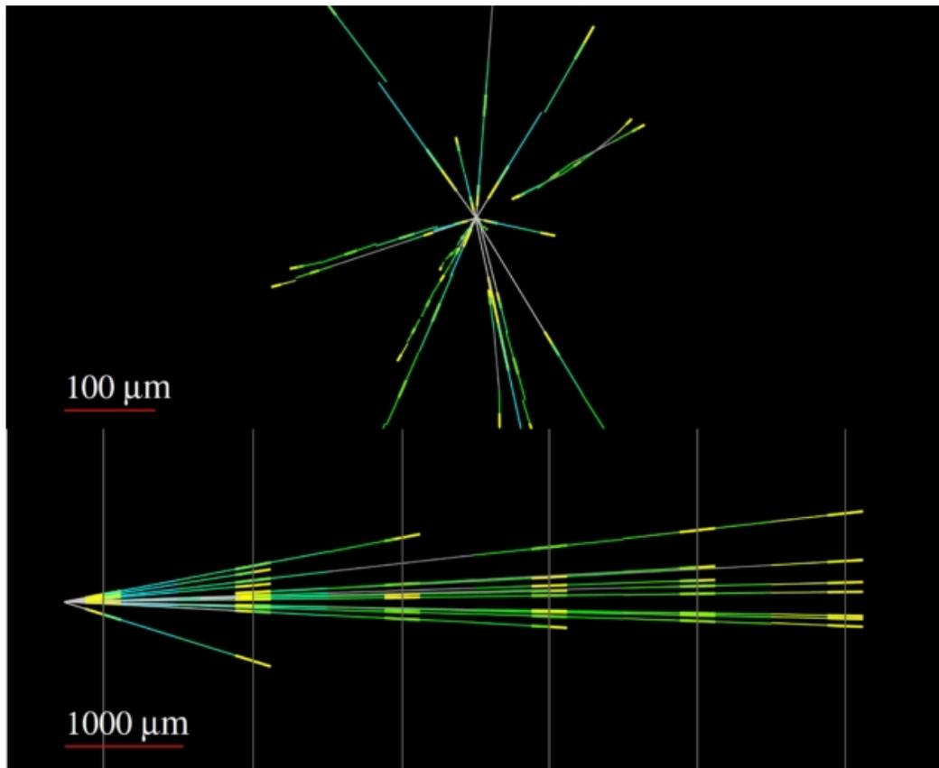
**New territory** Two candidate collider-neutrino events from the FASER $\nu$  pilot detector in the plane longitudinal to (top) and transverse to (bottom) the beam direction. The different lines in each event show charged-particle tracks originating from the neutrino interaction point. Credit: FASER Collaboration.
