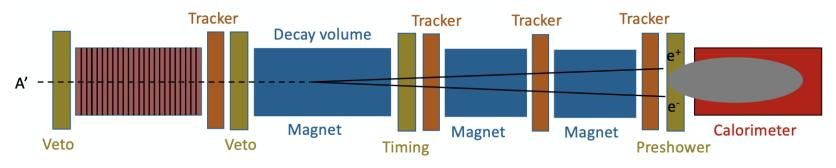
The signal is no charged particle passing through the upstream veto scintillator detectors, followed by two very energetic (100s of GeV – TeV) charged tracks in downstream trackers. Tracks are very collimated, but magnet splits them sufficiently to be seen as 2 tracks in trackers.
